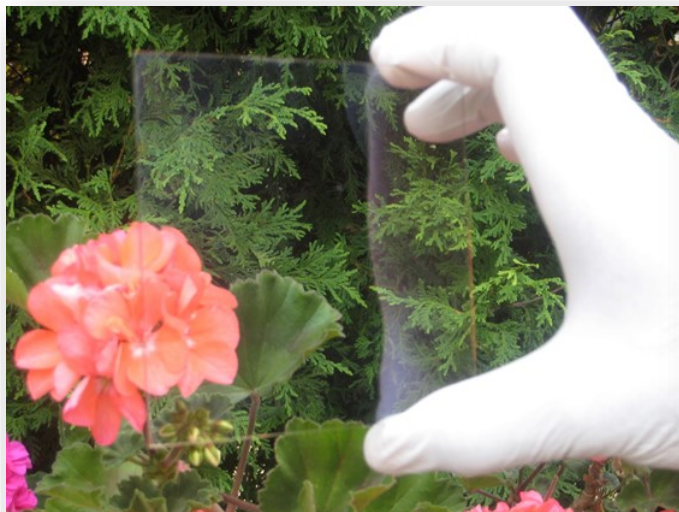
Sample of a high-transparency nano-thin diamond-like carbon based solar control coating on a glass substrate.
